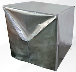
FabriCool is an advanced insulated packaging material specially designed to protect air cargo shipments against extreme ambient conditions. Made using a combination of a tough metalized outer layer and an internal fabric layer, FabriCool provides effective temperature control, while also allowing the contents to breathe to avoid build-up of condensation.
